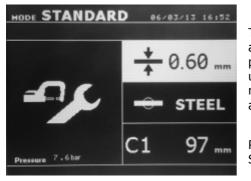
The skey is used to enter the clamp adjustment mode. The clamp adjustment mode allows the user to close the clamp and apply the programmed force on the electrodes without any current flowing. This mode is used to adjust the arms. The clamp will remain closed as long as the button remains pressed; this allows the user to check the alignment of the electrodes and positioning of the caps.
