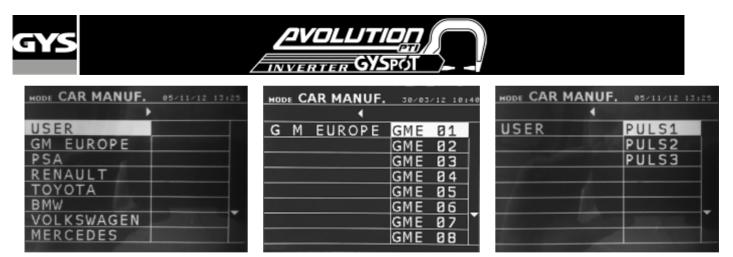
User programmed welding spots can be recalled by selecting USER in the list of car manufacturers. The welding spots can be programmed using the welding spot programming module in the GYSPOT software.
