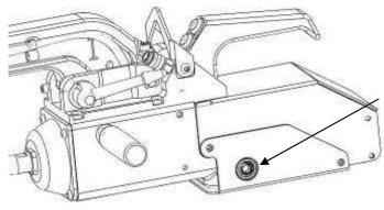
This screw fixes the copper cable terminals to the clamp. The tightening needs to be overhauled or you can have a loss of current or worst you can damage irreversibly your machine.
