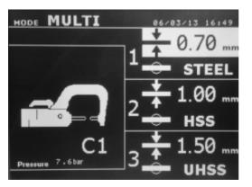
Using The up and down button (key definition diagram, (5)) allows selection of the parameters for each sheet. When the parameters for a sheet are highlighted, the sheet thickness and type of steel can be adjusted using the + and – keys (key definition diagram, (3)). The individual sheet parameters that can be adjusted in this mode are :
