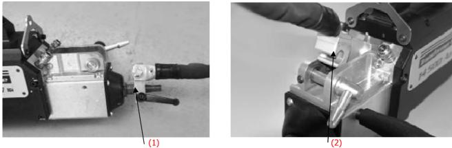
Select the clamp adjustment mode in the menus, in order to stop the pump and the flow of cooling liquid.Fix the earth cable on the removable electrode; put the clamp and tighten the lever.
