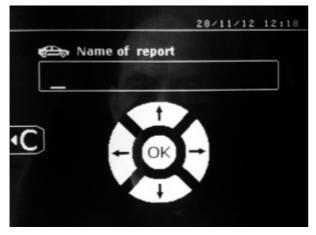
Saving a report allows spot welding data to be stored on a memory card, in order to retrieve it at a later date e.g. on a computer.
